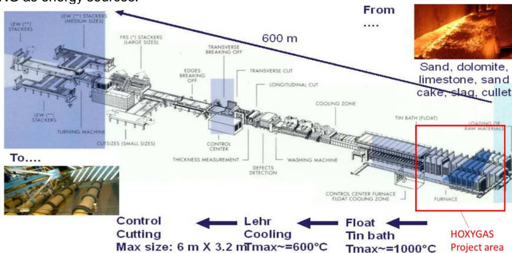
The HOxyGas project aimed at demonstrating the maturity and potential of the new technology by producing high quality automotive colour glass (which has higher quality requirements than architectural glass), using only natural gas as a combustible (more corrosive atmosphere, more foaming on glass surfaces).
